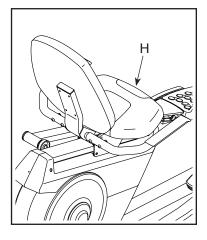
to the desired position, and then pull the adjustment handle inward to the center.
