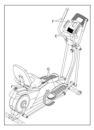
Push the pedals (G) until they begin to move with a continuous motion. Note: The pedals can turn in either direction. It is recommended that you move the pedals in the direction shown by the arrow; however, for variety, you can turn the pedals in the opposite direction.
