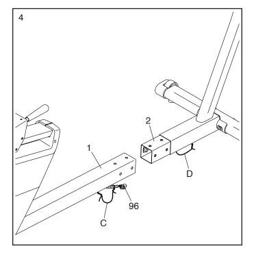
5. **Tip: Avoid pinching the wires.** Insert the Upright (2) into the Frame (1).
