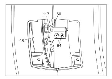
Next, rotate the Large Pulley (48) until a Pulley Magnet (117) is aligned with the Reed Switch (60). Slide the Reed Switch slightly toward or away from the Pulley Magnet. Then, retighten the M4 x 19mm Screws (84).
