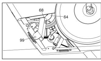
When the Drive Belt (64) is tight, tighten the M10 x 55mm Bolt (99). Then, reattach the side access cover.
